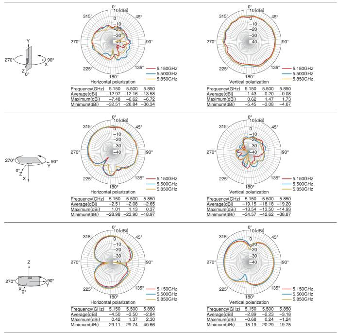
•Tested antenna has been soldered. Evaluation board size is 50x20x1 mm.
