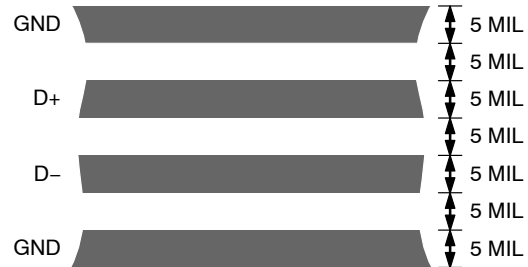
Figure 23. Typical Arrangement of Signal Tracks
