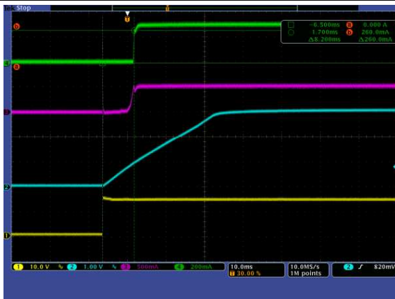
Ch1: Input voltage; Ch2: SS pin voltage; Ch3: Input current; Ch4: LED current; Time: 10 ms/div Figure 19. Soft-Start Sequence
