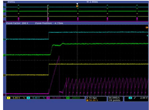
Ch1: DDRV voltage; Ch2: PWM input, TP3; Ch3: Switch sense current resistor (R15) voltage; Ch4: LED current; Time: 10 µs/div Figure 26. PWM Dimming (Duty cycle = 4%, Frequency = 240 Hz)
