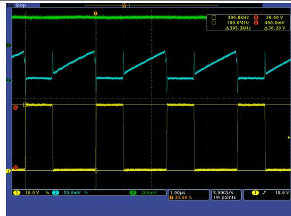
Ch1: Q2 Drain voltage; Ch2: Switch current sense (R15) voltage; Ch4: LED current; Time: 1 \mu s/div Figure 20. Nominal Operation
