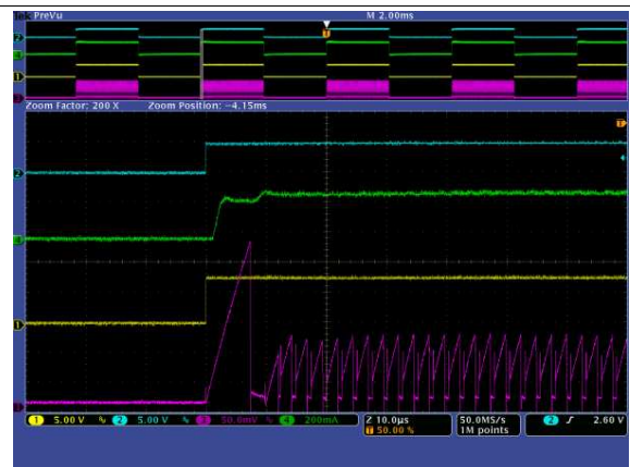
Ch1: DDRV voltage; Ch2: PWM input, Ch3: Switch sense current resistor (R15) voltage; Ch4: LED current; Time: 10 \mu s/div Figure 24. PWM Dimming (Duty cycle = 50 %, Frequency = 240 Hz)
