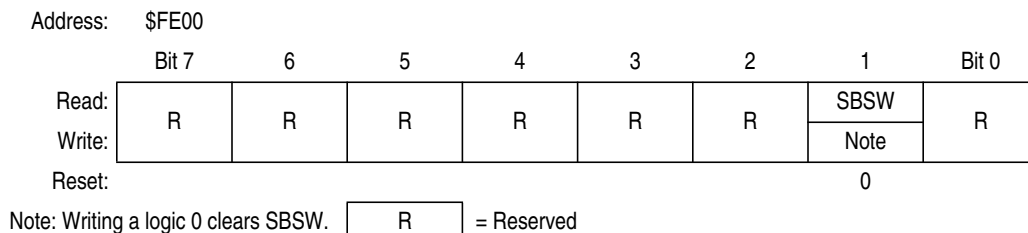
Figure 18-6. SIM Break Status Register (SBSR)
