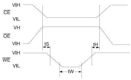
$$\begin{split} t_S &= t_H = 1 \; \mu \text{sec (min.)} \\ t_W &= 10 \; \text{msec (min.)} \\ V_H &= 12.0 \pm 0.5 \text{V} \end{split}$$
