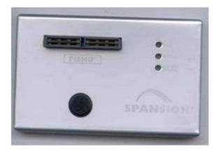
FSK-PUP (Flash Starter Kit – PISMO USB Programmer) is an advanced portable development tool that provides features including Read, Program, Erase, Burst Read, and Scripting of Cypress flash memories.
