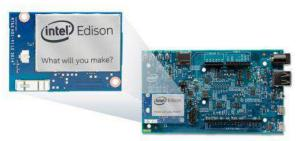
This kit includes an Arduino Breakout, which essentially gives your Edison the ability to interface with Arduino shields or any board with the Arduino footprint.
