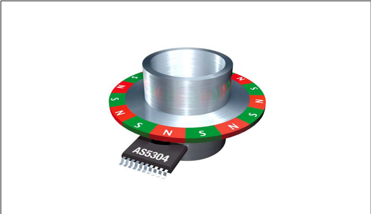
Figure 20: AS5304 (AS5306) with Multi-Pole Ring Magnet
