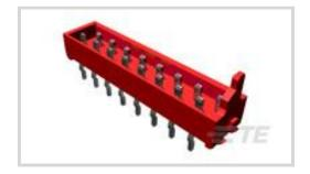
Connector System: Board-to-Board Number of Positions: 14 Centerline (Pitch): 1.27 mm [.05 in ] PCB Mount Retention: With PCB Mount Retention Type: Kinked Solder Tails All Male-on-Board Connector, Micro-MaTch (36)
