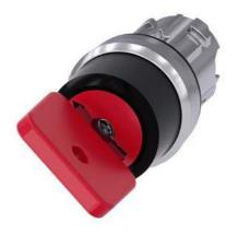
Key-operated switch O.M.R, 22 mm, round, metal, shiny, lock number 73037, red, with 2 keys, 2 switch positions O<I, momentary contact type, Actuating angle 45°, 10:30h/12h, key removal O, with laser labeling, upper case
