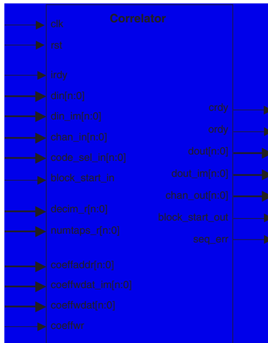
Figure 1. Correlator IP Core External Interface Diagram
