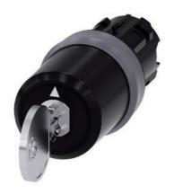
Key-operated switch BKS, 22 mm, round, plastic with metal front ring, lock number S1, with 2 keys, 3 switch positions I-O<II, left latching, right momentary contact type, actuating angle  $2x45^{\circ}$ , 10:30h/12h/13:30h, key removal I, with laser labeling, lower case
