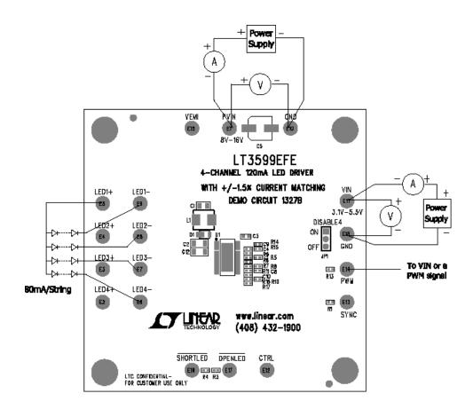
Figure 1. Proper Measurement Equipment Setup
