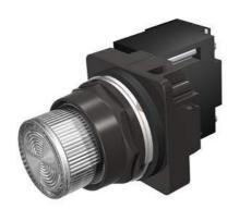
30mm BlackMax, Epoxy Coated Corrosion Resistant Complete Metal Unit Illuminated Indicator Light Transformer type, 240V AC LED Lamp, BA9s Plastic Lens, Clear UL Listed, CSA Certified NEMA 1,3,3R,4,4X,12,13 & Automotive Standards
