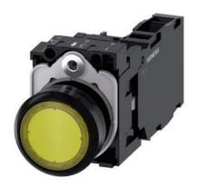
Illuminated pushbutton, 22 mm, round, plastic, yellow, pushbutton, flat, momentary contact type, with holder, 1 NO+1 NC, LED module with integrated LED 110 V AC, screw terminal
