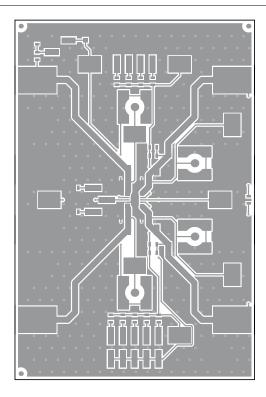
Figure 2. Top Layer Routing
