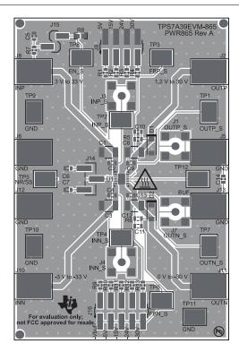
Figure 1. Assembly Layer
