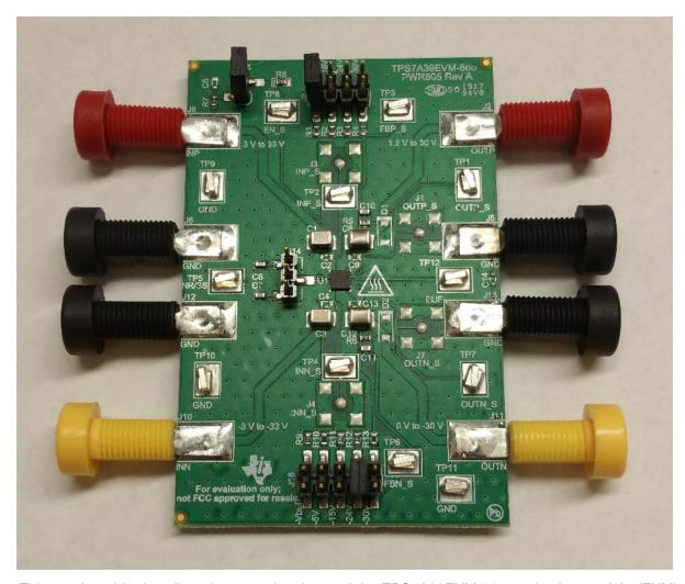
This user's guide describes the operational use of the TPS7A39EVM-865 evaluation module (EVM) as a reference design for engineering demonstration and evaluation of the TPS7A3901DSC, low-dropout linear regulator (LDO). Included in this user's guide are setup and operating instructions, layout guidelines, a printed circuit board (PCB) layout, a schematic diagram, and a bill of materials (BOM).
