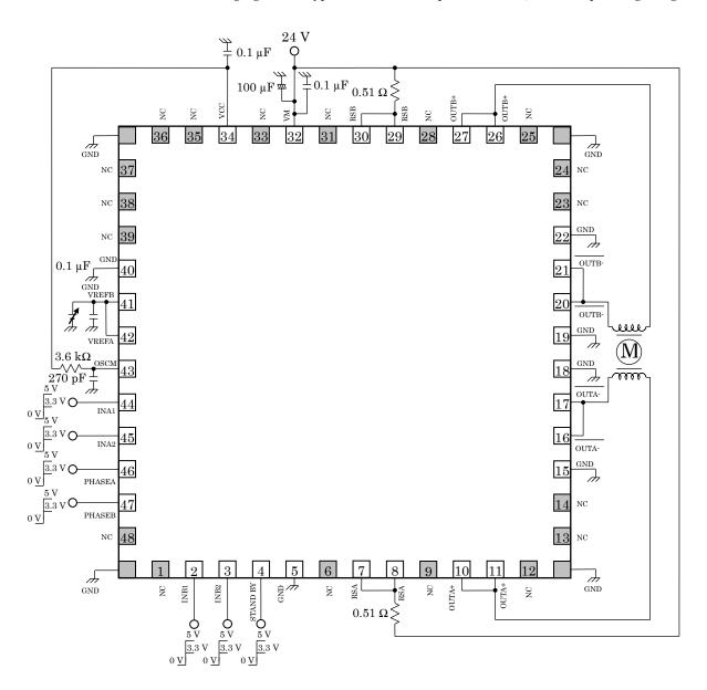
Note: I will recommend the addition of a capacitor if necessary. The GND wiring must become one point as much as possible-earth.
