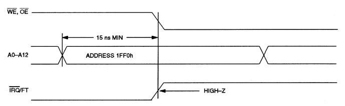
The IRQ/FT pin can also be activated in the battery-backed mode. The IRQ/FT will go low if an alarm occurs and both ABE and AE are set. The ABE and AE bits are cleared during the power-up transition, however an alarm generated during power-up will set AF. Therefore the AF bit can be read after system power-up to determine if an alarm was generated during the power-up sequence. Figure 4 illustrates alarm timing during the battery backup mode and power-up states.
