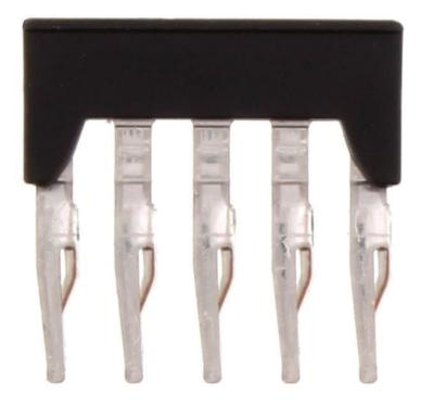
Insulated cross-connector, No. of poles: 5, Mounting type: Plug in, Width: 24.4 mm, Rated cross-section: 2.5 mm<sup>2</sup>, Colour: Black
