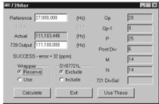
Figure 13. Generating 111.1MHz Without the Wrapper
