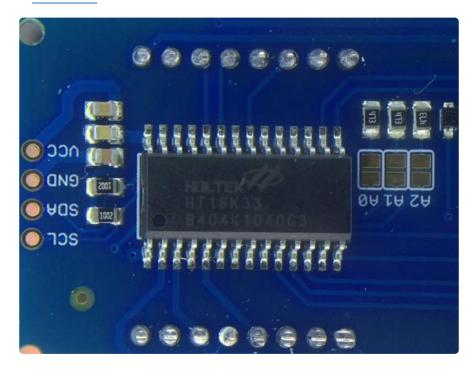
It's a wonderful chip! Not only is it capable of driving a 16x8 LED Matrix, but reading a pushbutton matrix with a maximum size of 13x3. In fact, this is how HT16K33 is used on the Adafruit Trellis (http://adafru.it/1616) to read the 16 pushbuttons.
