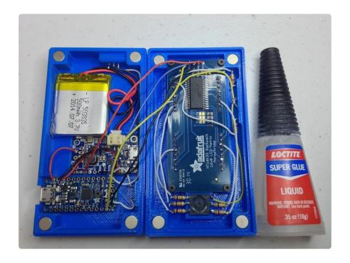
Finally use some super glue to secure the eight magnets to the cavities on the enclosure. Wait for a little bit to allow the glue to dry completely.
