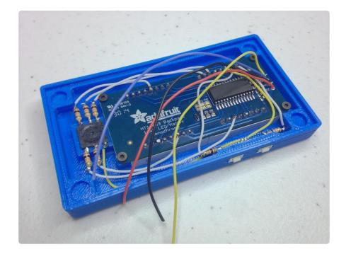
Solder four wires to the I2C pins on the Backpack. The colors I used in the picture above are the same as the ones in the circuit diagram on the previous page.
