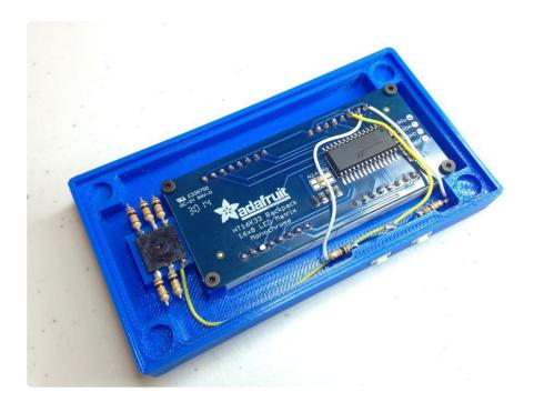
Solder the two white wires from the pushbutton resistors to the 1st and 2nd pins on the left side of the top LED matrix.
