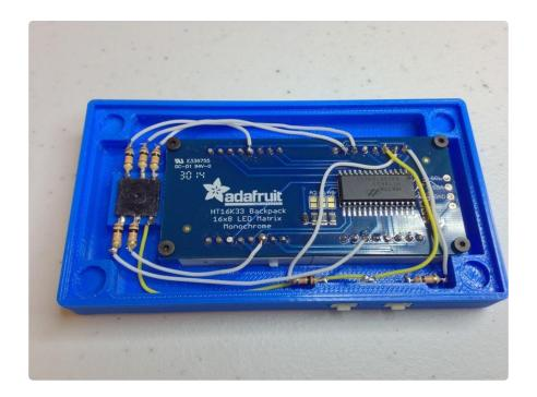
Then we can solder the last set of wires to connect the two resistors on the right side of the joystick to the backpack. Again, please refer to the circuit diagram on the previous page if the picture looks confusing.
