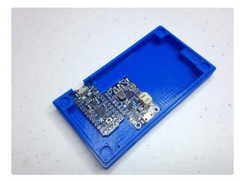
Start by putting the Pro Trinket and the PowerBoost 500 Charger into the enclosure. Use a M2 screw to secure the Pro Trinket. Gently push the PowerBoost into the cavity to fix it in place. It should be more or less a friction fit.
