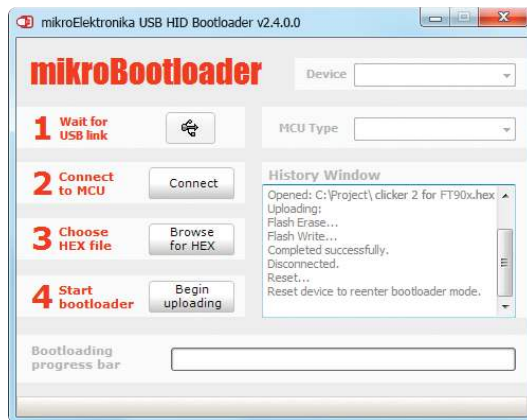
Figure 3-8: mikroBootloader ready for next job
