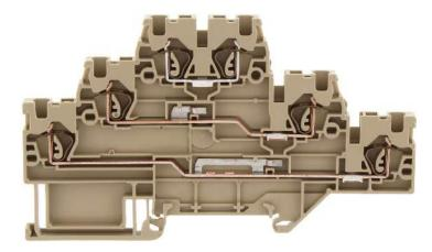
Three-level initiator terminal | Multi-wire terminal, Tension-spring connection, Mounting type: Mounting rail TS 35/7.5, Rated cross-section: 2.5 mm<sup>2</sup>, Width: 5.1 mm, Colour: Beige
