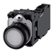
Illuminated pushbutton, 22 mm, round, plastic, clear, pushbutton, flat, momentary contact type, with holder, 1 NO+1 NC, LED module with integrated LED 230 V AC, screw terminal
