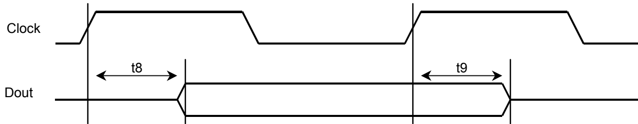
Figure 18-5. To/From High-Z Delay Definitions (Rising Clock Edge)
