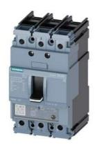
circuit breaker 3VA5 UL frame 125 breaking capacity class S 25kA @ 480 V 3-pole, line protection TM230, FTAM, In=80A overload protection Ir=80A fixed short-circuit protection Ii=5...10 x In UL489 SB (naval), 50 deg. cel. cable connection on both sides
