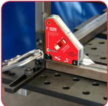
NOTE: Must be used for tack welding only and removed before completing weld. Avoid prolonged exposure of magnetic products to heat sources of 356°F / 180°
