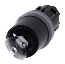
Key-operated switch IKON, 22 mm, round, plastic with metal front ring, lock number 360012K1, with 2 keys, 2 switch positions O-I, latching, actuating angle  $90^\circ, 10:30h/13:30h$ , key removal O+I, with laser labeling, upper case and lower case, always upper case at beginning of line
