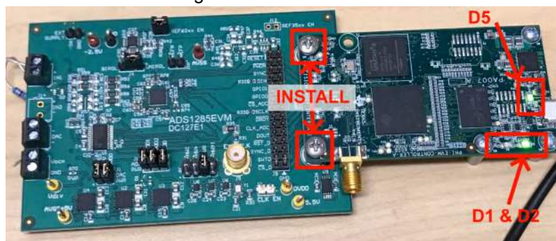
Figure 2-1. ADS1285EVM-PDK Hardware Setup and LED Indicators
