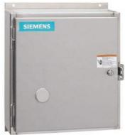
Electrically held lighting contactor, Contactor amp rating 30A, 0 N.C. / 3 N.O. Poles, 220VAC 50HZ/240VAC 60HZ coil, Non-combination type, (no disconnect device), Encl NEMA type 4X 304 S-Steel, Water/dust tight noncorrosive
