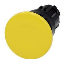
Mushroom pushbutton, 22 mm, round, plastic, yellow, 40mm, momentary contact type, with laser labeling, upper case and lower case, always upper case at the beginning of the word
