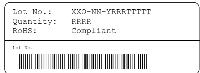
Figure 22: First label on reel: XX = Sensor Type (21 for SHT21), O = Output mode (D = Digital, P = PWM, S = SDM), NN = product revision no., Y = last digit of year, RRR = number of sensors on reel divided by 10 (200 for 2000 units), TTTT = Traceability Code.
