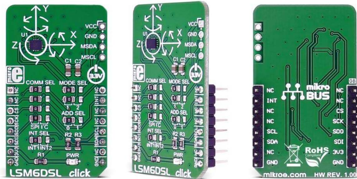
**LSM6DSL click** measures linear and angular velocity with six degrees of freedom. It carries the LSM6DSL high-performance 3-axis digital accelerometer and 3-axis digital gyroscope. The click is designed to run on a 3.3V power supply. LSM6DSL click communicates with the target microcontroller over SPI or I2C interface, with additional functionality provided by the INT pin on the mikroBUS™ line.
