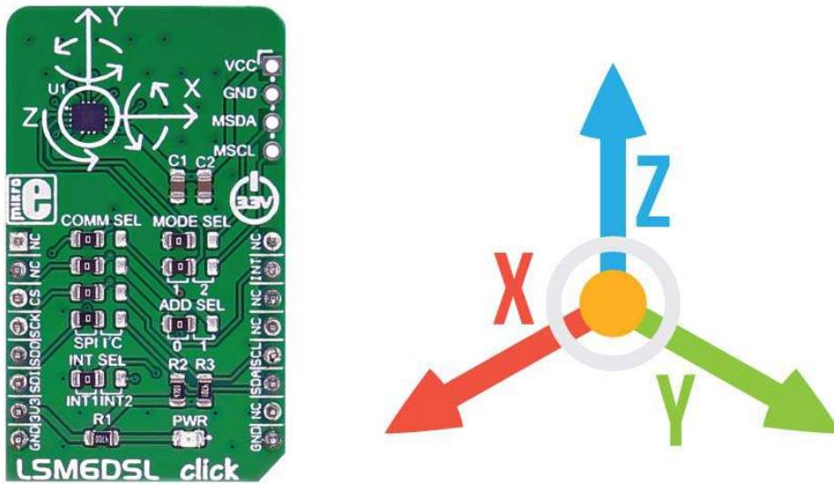
The event-detection interrupts enable efficient and reliable motion tracking and contextual awareness, implementing hardware recognition of free-fall events, 6D orientation, click and double-click sensing, activity or inactivity, and wakeup events
