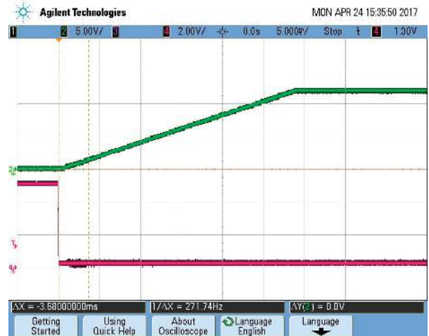
Figure 12. Vin Start-up Delay (CH2: Vout, CH1: Vin) (Vin=48V, Iout=50A, Cload=330µF, Ta=+25°C, 20ms/div)
