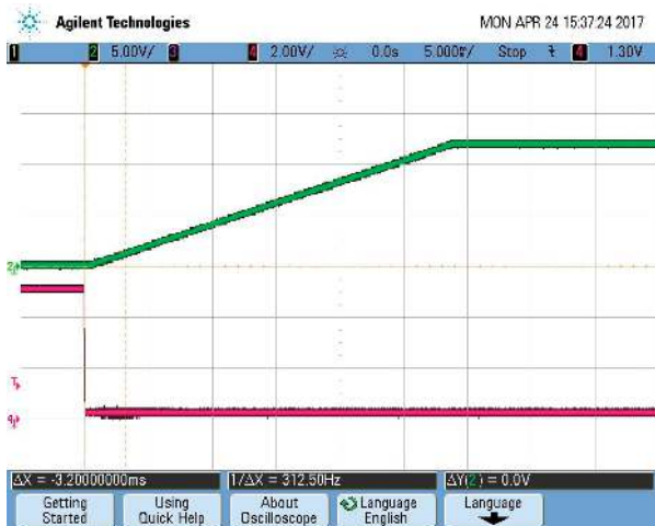
Figure 11. Vin Start-up Delay (CH2: Vout, CH1: Vin) (Vin=48V, Iout=0A, Cload=330µF, Ta=+25°C, 20ms/div)
