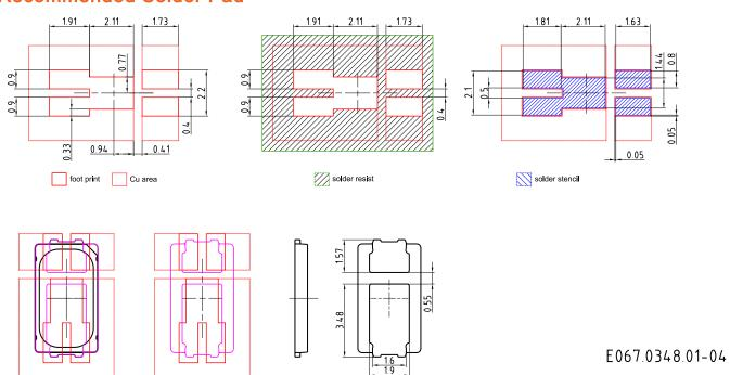
For superior solder joint connectivity results we recommend soldering under standard nitrogen atmosphere. Package not suitable for ultra sonic cleaning.
