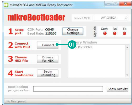
Figure 3-5: Connecting with mikroBootloader
