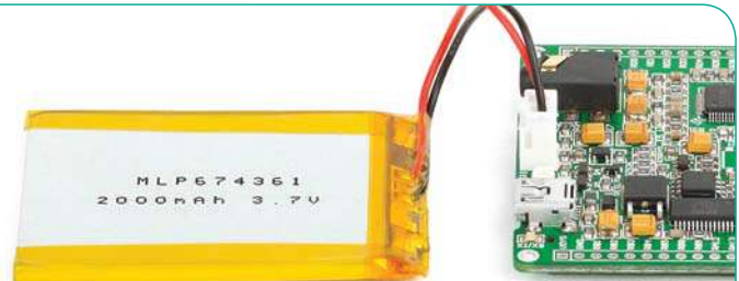
Figure 1-2: Connecting Li-Polymer battery
