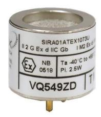
If a flammable gas is present when the bead is heated to about 400 to 500  $^{\circ}$ C, the gas will oxidise and the resultant release of energy will heat the bead still further. This increase in temperature is detected as an increase in resistance of the coil.
