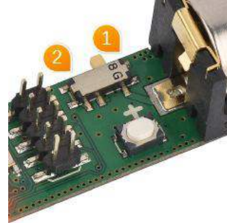
Figure 5. Power Supply Switch. Position 1 – Battery Powered Operation, Position 2 – Debug Link Connector Powered Operation
