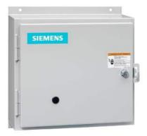
Reversing NEMA contactor Size 0 Single phase full voltage Contactor amp rating 18Amp 3 w 110-120/220-240VAC 60HZ coil Non-combination type Enclosure NEMA type 12 Dust/drip proof for indoors Standard width enclosure
