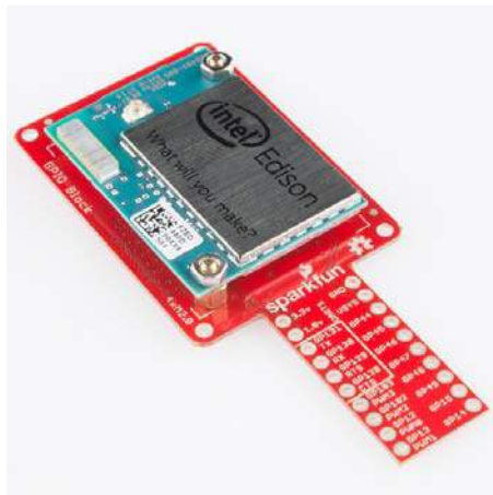
GPIO Block Installed
