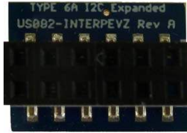
Figure 3. US082-INTERPEVZ Pmod Board (Top)
