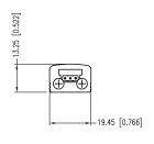
\*UNLESS OTHERWISE SPECIFIED TOLERANCES PER DECIMAL PRECISION ARE: X=±1 (±0.039), X.X=±0.5 (±0.020), X.XX=±0.25 (±0.010), X.XXX=±0.127 (±0.005). LEAD SIZE=±0.05 (±0.002), LEAD LENGTH=±0.75 (±0.030). MIN=  $^{+DECIMAL}_{-0.00}$  PRECISION MAX.=  $^{+0.00}_{-DECIMAL}$  PRECISION
