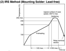
(The temperature profile indicates the temperature on the PCB.)
