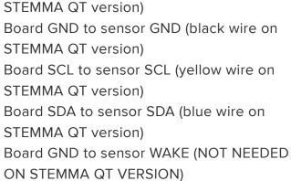
Board 3V to sensor VIN (red wire on
