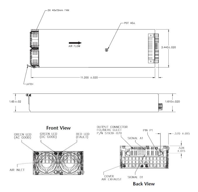
Input: 90V<sub>AC</sub> to 264V<sub>AC</sub>; Output: 48V<sub>DC</sub> @ 1200W; 5 V<sub>DC</sub> @ 0.5A
