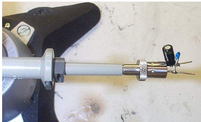
Figure 35 – Oscilloscope Probe with Probe Master ( www.probemaster.com ) 4987A BNC Adapter. (Modified with wires for ripple measurement, and two parallel decoupling capacitors added)
