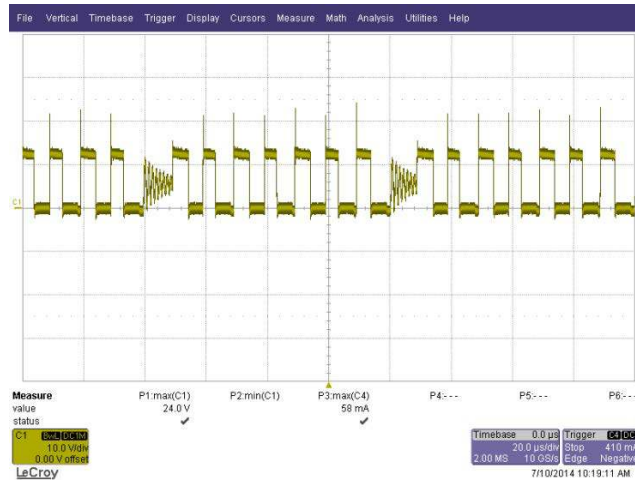
Figure 32 – SR FET Voltage Waveforms. 85 VAC Input, 2 A Load. V_{DRAIN} , 10 V, 20 \mu s / div.
