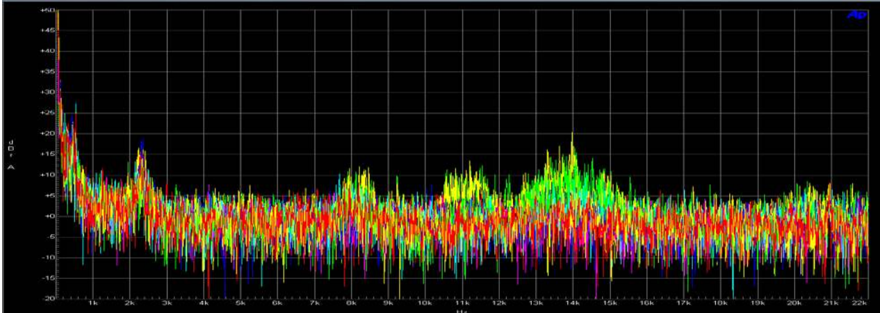
Figure 49 – Audible Noise Spectrum: 265 VAC, I_{OUT} Swept from 0 A to 2.0 A.
