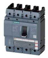
circuit breaker 3VA5 UL frame 250 breaking capacity class C 100kA @ 480V 4-pole, line protection TM230, FTAM, In=100A overload protection Ir=100A fixed short-circuit protection Ii=5...10 x In N conductor unprotected without connection
