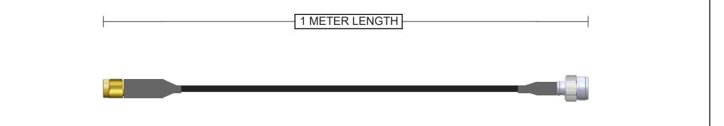
Connector A 132451 SMA Plug Straight Brass Gold + Heatshrink 50 Ohm LMR-240 Continuity/Hi-Pot Connector B 031-6825 TNC Plug Straight Brass Nickel + Heatshrink
