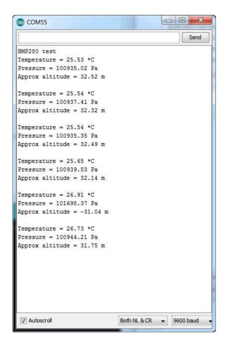
Temperature is calculated in degrees C, you can convert this to F by using the classic F = C \* 9/5 + 32 equation.
