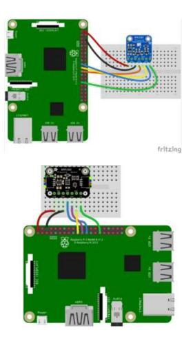
Pi 3V3 to sensor VIN Pi GND to sensor GND Pi MOSI to sensor SDI Pi MISO to sensor SDO Pi SCLK to sensor SCK Pi #5 to sensor CS (or use any other free GPIO pin)
