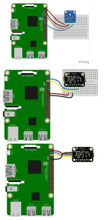
Pi 3V3 to sensor VIN (red wire on STEMMA version) Pi GND to sensor GND (black wire on STEMMA version) Pi SCL to sensor SCK (yellow wire on STEMMA version) Pi SDA to sensor SDI (blue wire on STEMMA version)
