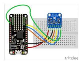
Board GND to sensor GND Board SCK to sensor SCK Board MOSI to sensor SDI Board MISO to sensor SDO Board D5 to sensor CS (or use any other free digital I/O pin)
