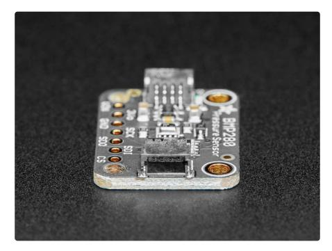
Nice sensor right? So we made it easy for you to get right into your next project. The surface-mount sensor is soldered onto a custom made PCB in the <u>STEMMA QT form</u> factor (), making them easy to interface with. The <u>STEMMA QT connectors</u> () on either side are compatible with the <u>SparkFun Qwiic</u> () I2C connectors. This allows you to make solderless connections between your development board and the BMP280 or
