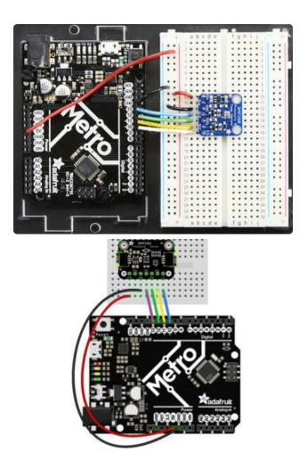
Connect Vin to the power supply, 3V or 5V is fine. Use the same voltage that the microcontroller logic is based off of. For most Arduinos, that is 5V Connect GND to common power/data ground Connect the SCK pin to Digital #13 but any pin can be used later Connect the SDO pin to Digital #12 but any pin can be used later Connect the SDI pin to Digital #11 but any pin can be used later Connect the CS pin Digital #10 but any pin can be used later
