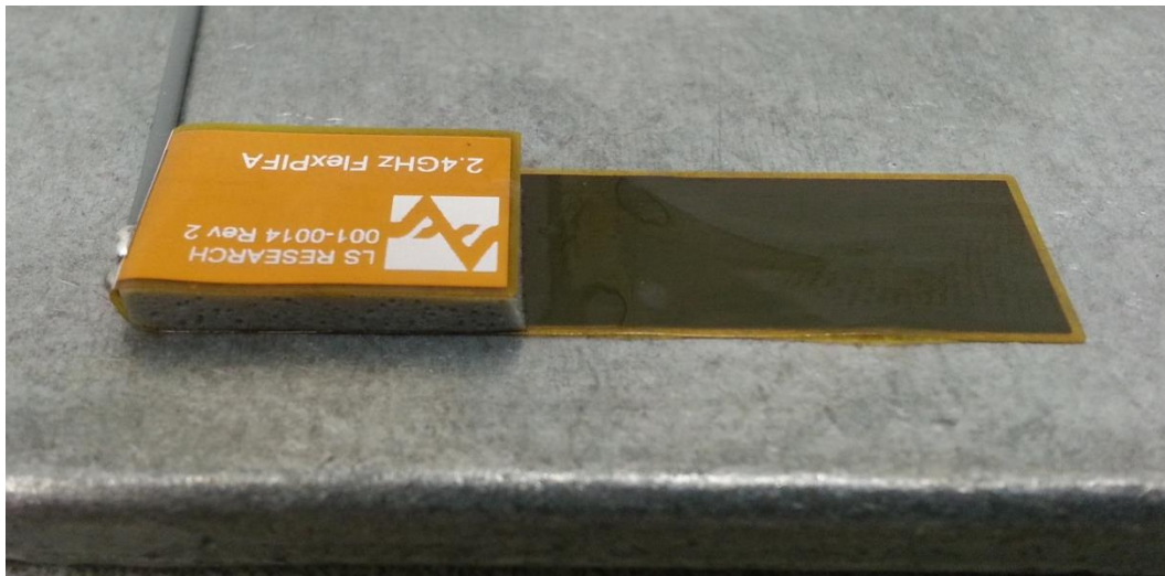
Figure 24 FlexPIFA Mounted on Metal
