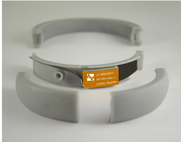
Figure 27 FlexPIFA Integrated into Bracelet
